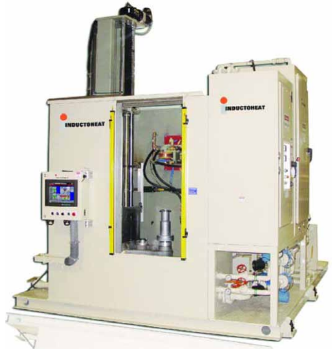
Figure 5 Inductoheat's simultaneous dual-frequency inverter for gear contour hardening (courtesy Inductoheat).
