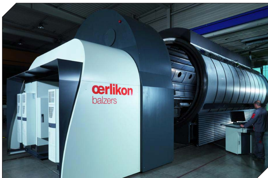
Figure 2 In the PPD chamber, parts with a weight of up to 40 metric tons and dimensions of 32.2 ft. × 8.9 ft. × 5 ft. can be processed.
