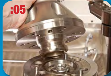
Install a new Quick-Flex®Plus module onto the common workholding interface.
