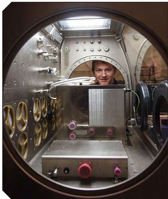
Made In Space CEO Aaron Kemmer stares through the windows of the Microgravity Science Glovebox with the Zero-G 3D Printer enclosed (Photo: Made In Space).
