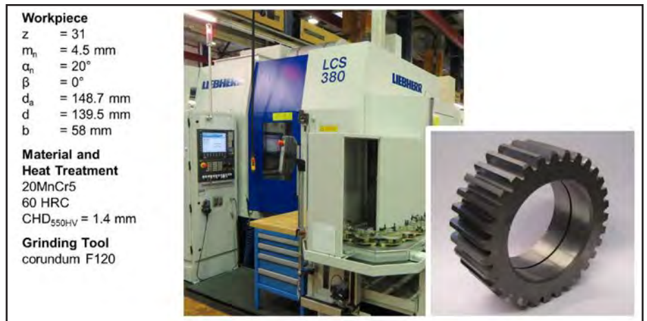
Figure 3 Workpiece data and machine tool.
