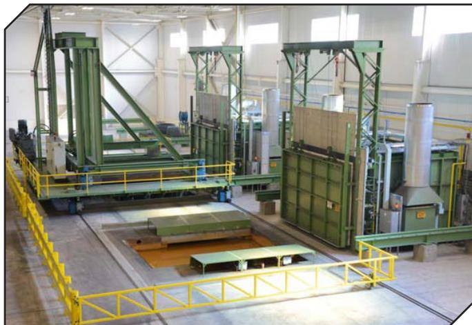
McInnes Rolled Rings has completed an \$8 million, 25,000-square-foot expansion to its current manufacturing facility. The addition expands its present heat treat size capabilities by providing the ability to quench and temper forgings up to 144 inches in diameter. With separate high agitation water and polymer quench tanks, this new state-of-the-art bay will significantly expand the daily tonnage capacity to ensure the fastest delivery times available in the industry.
