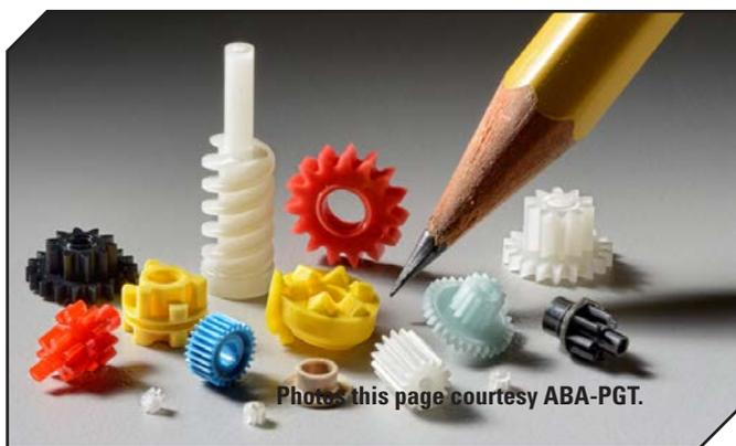
“Design can also affect gear performance. For example, the gear designer should take advantage of the fact that a custom gear mold must be cut to account for shrinkage variations by modifying gear teeth beyond standard proportions to increase contact ratios and load sharing. Additionally, full-round gear tooth roots should always be used to minimize stress concentrations and molded-in stresses that can compromise gear performance. Molding can likewise affect plastic gear performance.
