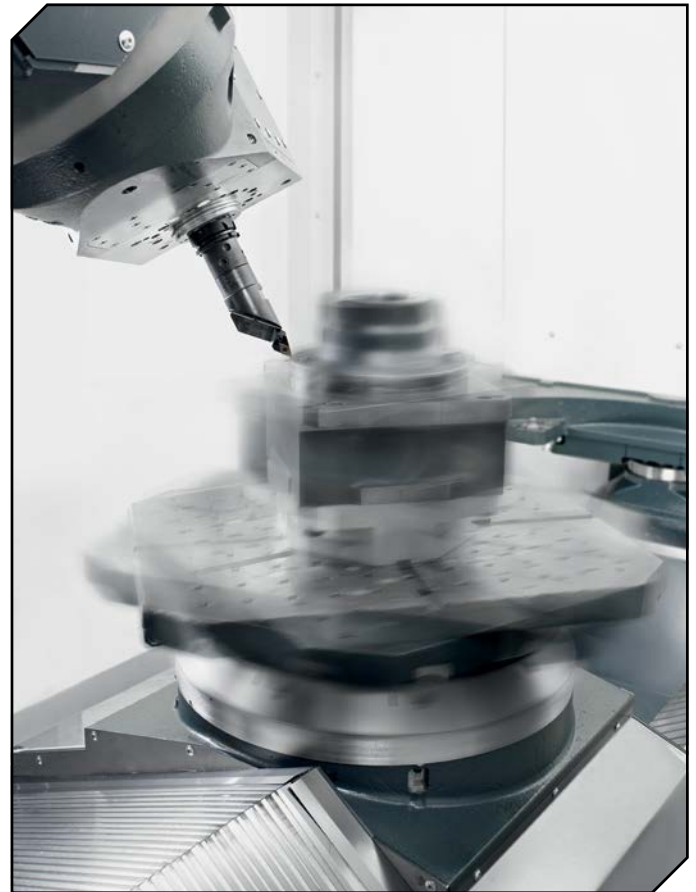
Figure 7 Even true turning operations can be performed on C-type machines equipped with high-speed worktables.
