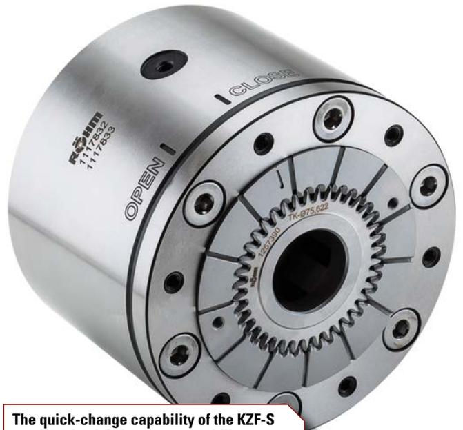
Global Gear is a Downers Grove, Illinois-based manufacturer serving Tier 1 and Tier 2 diesel engine OEMs and other engine manufacturers in the broad automotive and construction/agriculture industries. Their choice of workholding is the KZF-S collet chuck from Röhms, an external clamping chuck designed specifically for surface face grinding and hard turning gears.
