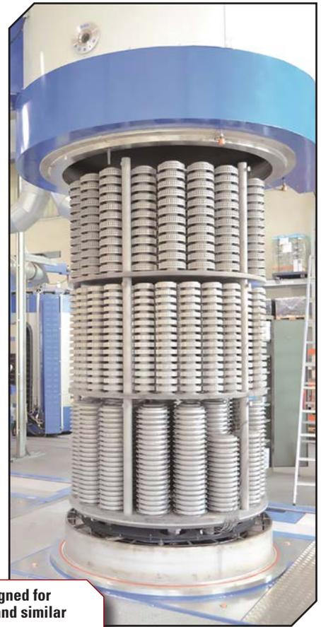
Rübzig's Mircopuls Everest system is designed for plasma nitriding gears, shafts, bearings and similar parts (image courtesy of Rübzig)
