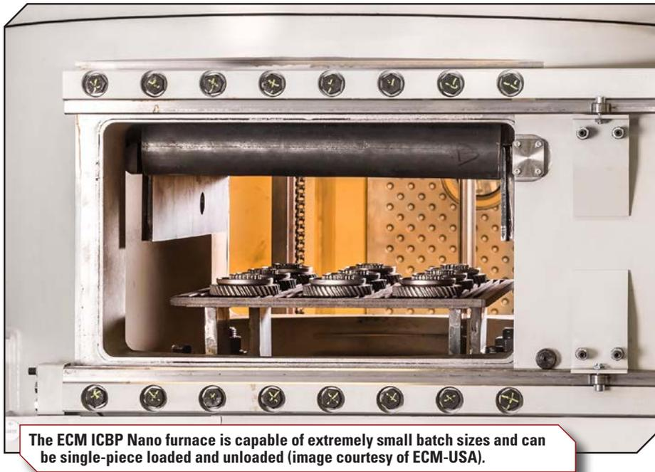
The ECM ICBP Nano furnace is capable of extremely small batch sizes and can be single-piece loaded and unloaded (image courtesy of ECM-USA).
