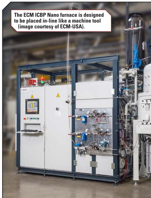
The ECM ICBP Nano furnace is designed to be placed in-line like a machine tool (image courtesy of ECM-USA).
