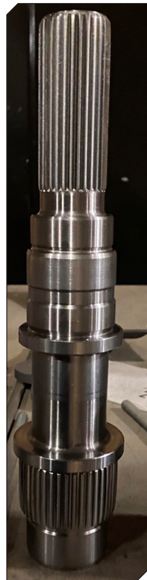
Figure 6 For vertical applications and oil quenching, precision positioning of parts like shafts is critical.
