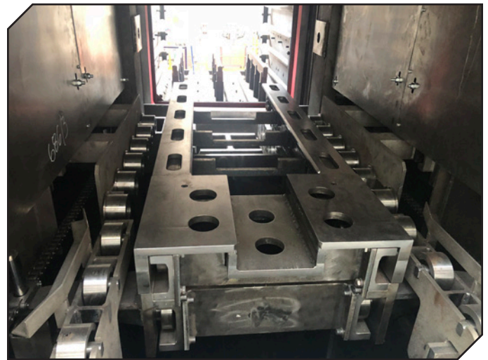
Figure 3 Precision internal furnace fork loading for oil quenching compatible with CFC trays.
