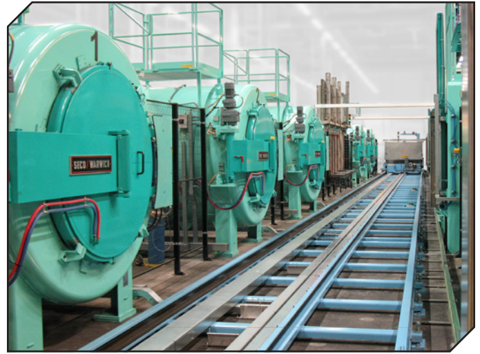
Figure 2 Furnace for nitriding and ferritic nitrocarburizing (photo courtesy of Seco/Vacuum Technologies).
