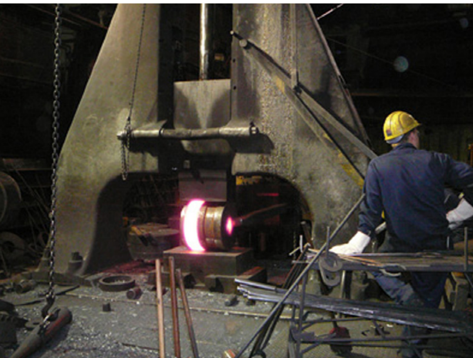
To optimize efficiency and reduce costs, rings and other parts can be produced for the wind power and energy industry as near-net-shaped forged parts with more refined surface finishes.
