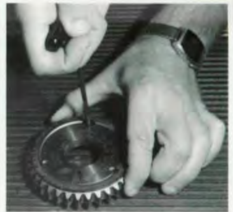
Fig. 6—Easy assembly and disassembly using three screws.
