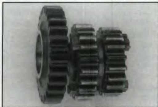
Fig. 4 — Wear of motorcycle gear after oil leakage during a race. Right: uncoated. Left: WC/C-coated.
