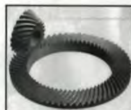
Fig. 3 — Spiral bevel gear set modeled as described in text.
