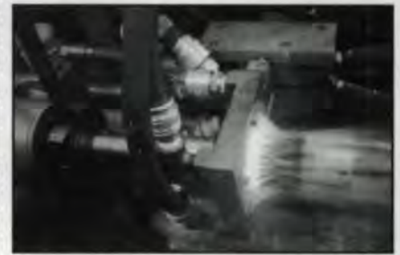
Fig. 1 — Machined integral quench coil with quick disconnect for power, water and quench.
