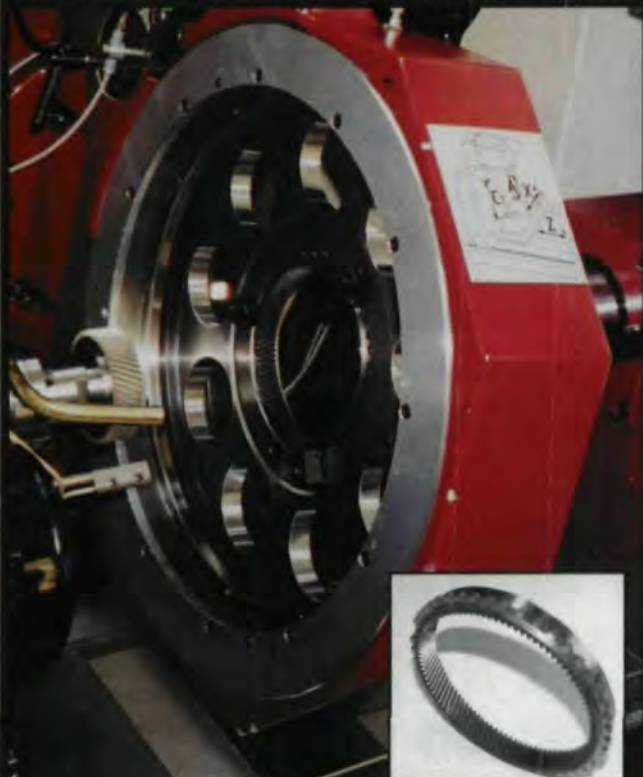
Honing of Automatic Transmission Ring Gear
