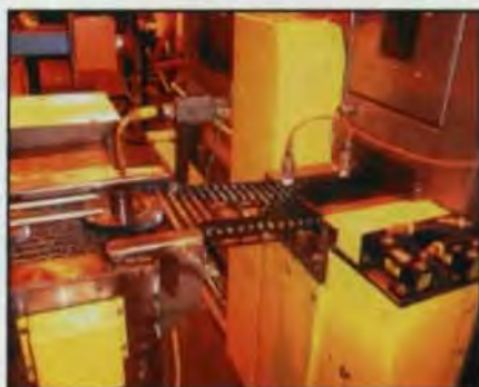
Universal Ice Blast built the machine, its first ice-blast gear-cleaning system, for Ford Motor Co. The Ford plant in Sharonville, OH, is using the machine to clean the input transfer gear used in the transmission of the Ford Focus.
