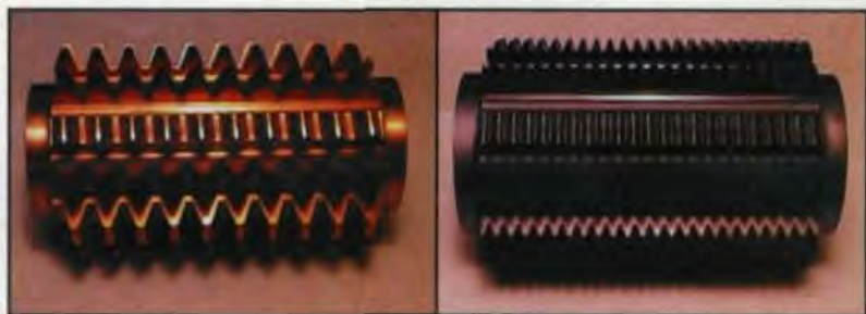
Figure 6—K-grade, TiN-coated carbide hob (left) and P-grade, TiAlN-coated carbide hob.
