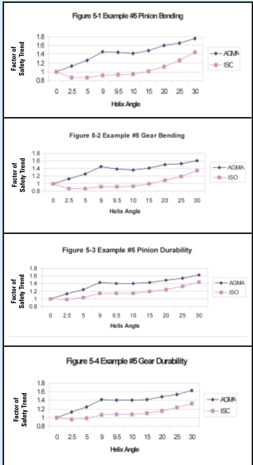
safety for both the pinion and the gear are lower for a helical gear than for a spur gear until the helix angle reaches 15° on this sample gear set. In AGMA, the factors of safety for bending on both the pinion and the gear in this gear set are lower between the value for the helix angle that has a helical overlap greater than 1.0 and a helix angle of 15°.
