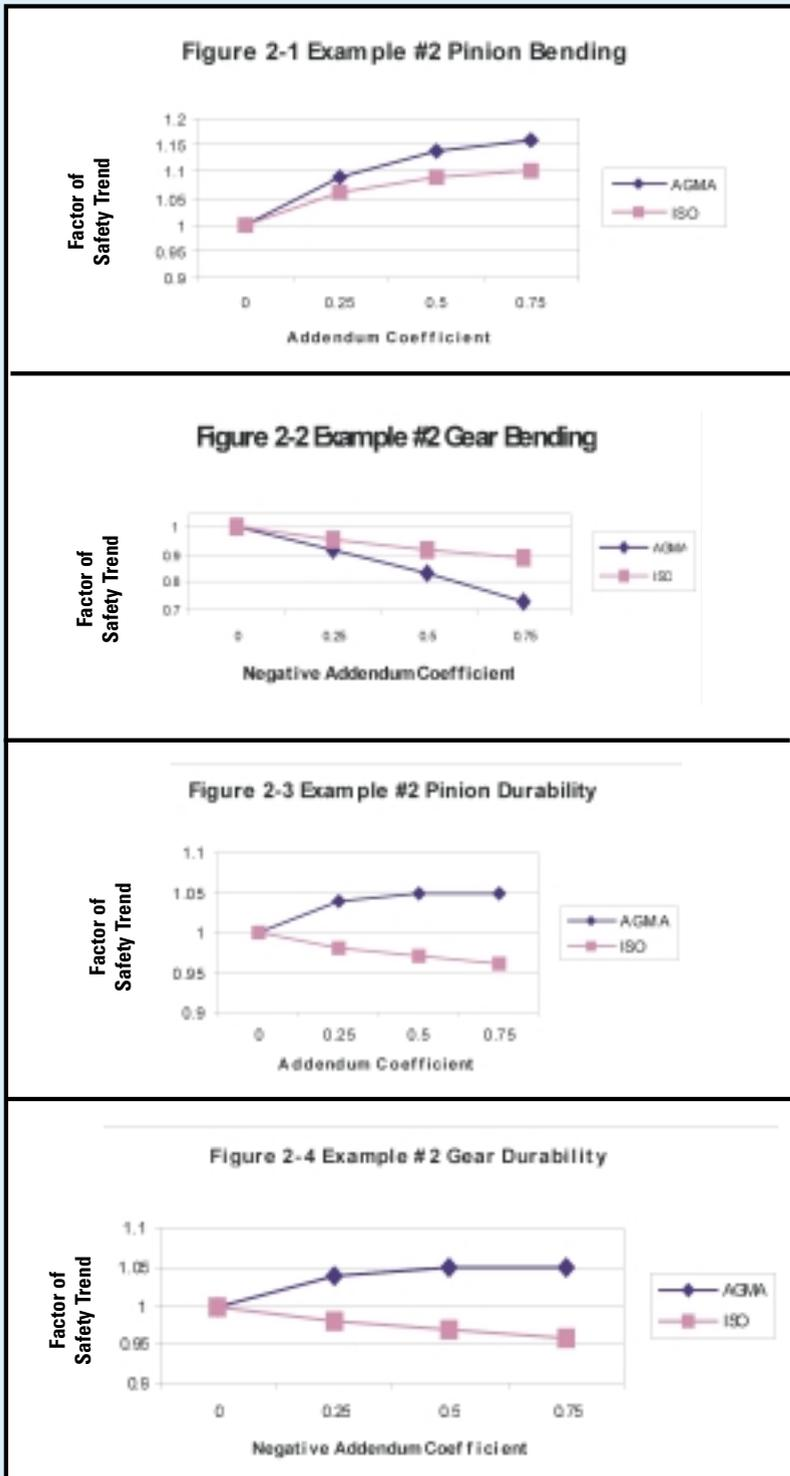
Even though there is a negative addendum modification on the gear, both AGMA and ISO give an increase in the factors of safety for durability on this spur gear. The factor of safety is increasing with the growing value of negative addendum modification coefficient. The increases in the factors of safety are higher in AGMA than they are in ISO.
