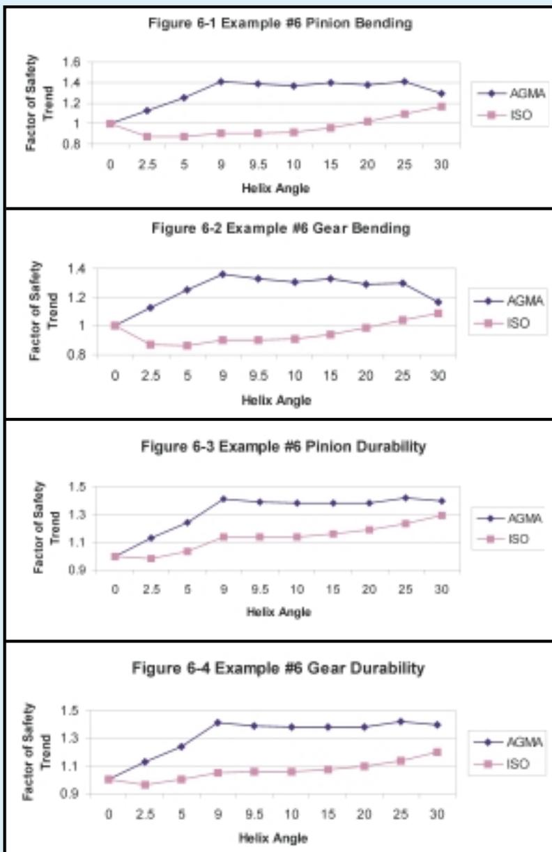
at a steeper slope with an increase in the helix angle. In ISO, the factor of safety for a helical gear is less than that of a spur gear until the helix angle is greater than 20°. In ISO, the factor of safety increases with an increasing helix angle if you do not consider the spur gear case. Above a 15° helix angle, the ISO factor of safety increases as the helix angle is increased and at a steeper slope.
