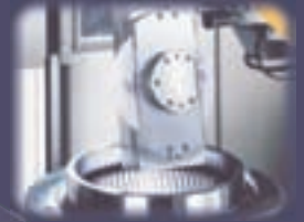
Internal grinding with dressable grinding wheels and measuring probe arm.
