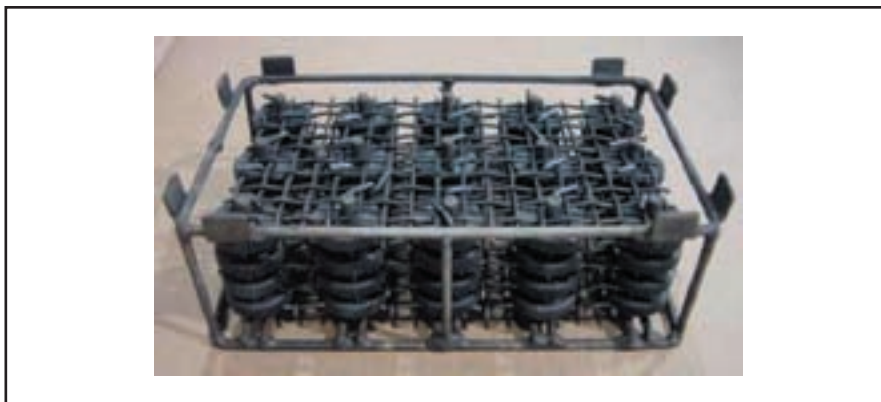
Figure 7—Gear heat treat baskets.
