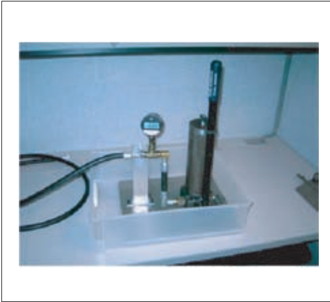
Figure 3—Manually operational hydraulic pump used to load gears (plastic container is for spill containment).
