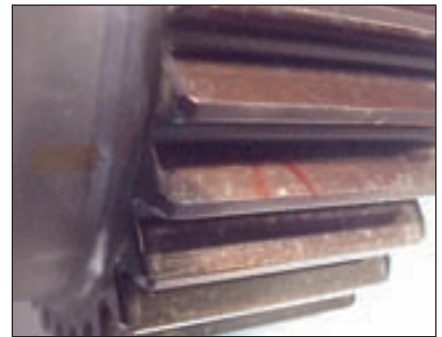
Figure 2—FOD on spur pinion.
