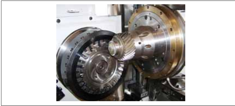
Figure 6—Hypoloid pinion cutting.
