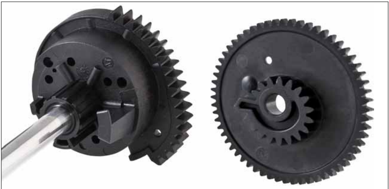
Non-circular gear segments where corrective action was successfully applied by Dontyne Systems (courtesy of Dontyne).
