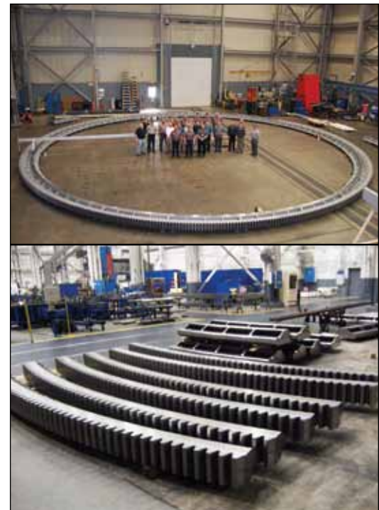
MAG cut 588 teeth in a 19-meter gear assembly using dedicated fixtures and special tooling (courtesy of MAG).
