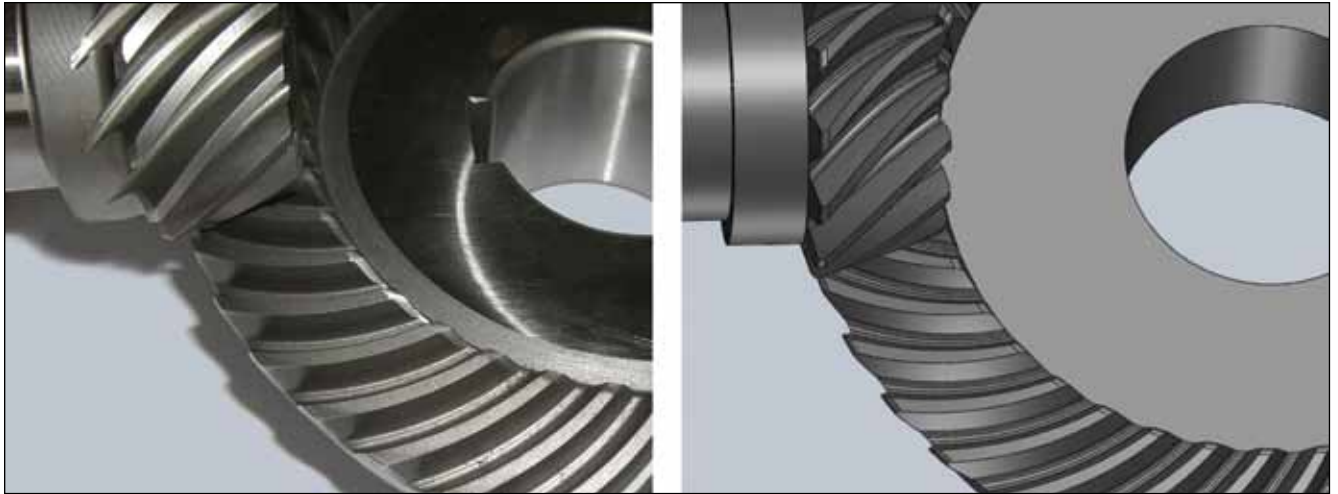
This bevel gear set was reproduced using software from GWJ Technology (courtesy of GWJ).
