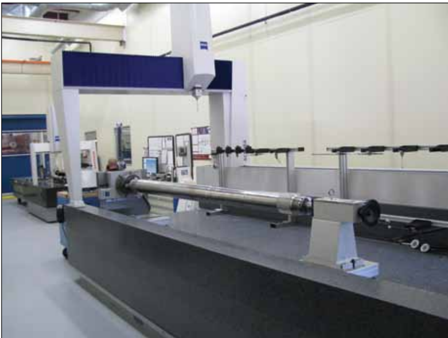
A 4.2 meter Accura with Vast XT gold sensor measures a turbine shaft with gears (courtesy of Carl Zeiss).
