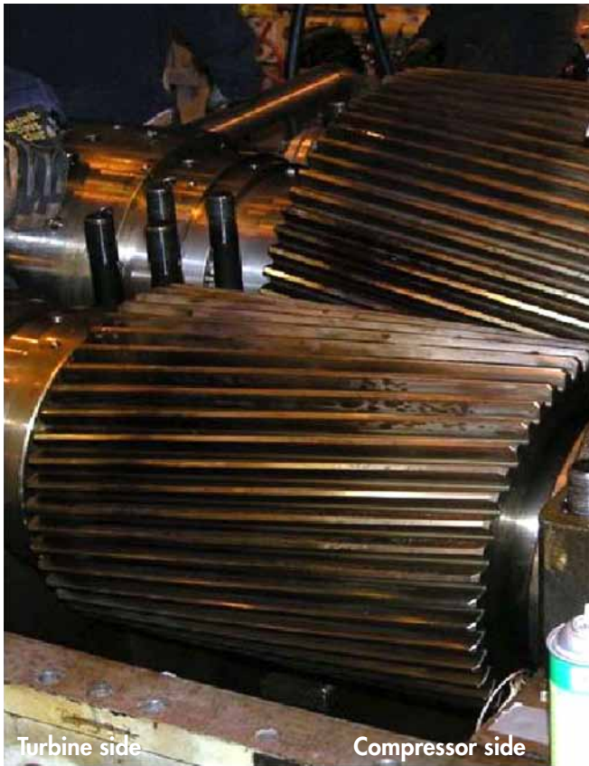
Figure 5—Varnish deposits on gear teeth.
