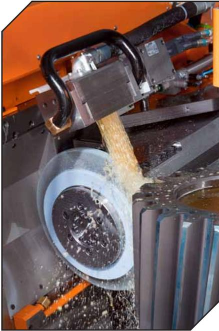
material for this wear-optimized grinding is no longer left to wear-out on the tip; as a result the risk of grinder-burn is minimized, and the workpiece is protected. Number of strokes and production time can be reduced as a result, depending on application.
