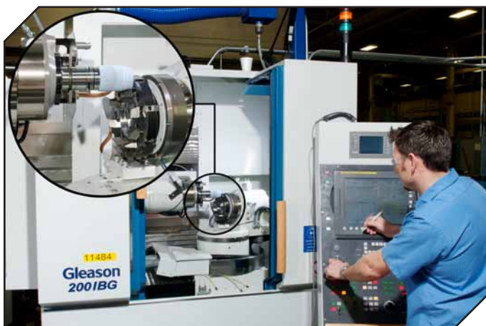
A single Gleason IBG (inserted blade grinder) out-performs many older manual grinders, raising quality and productivity on inserted blade production to unprecedented new levels.
