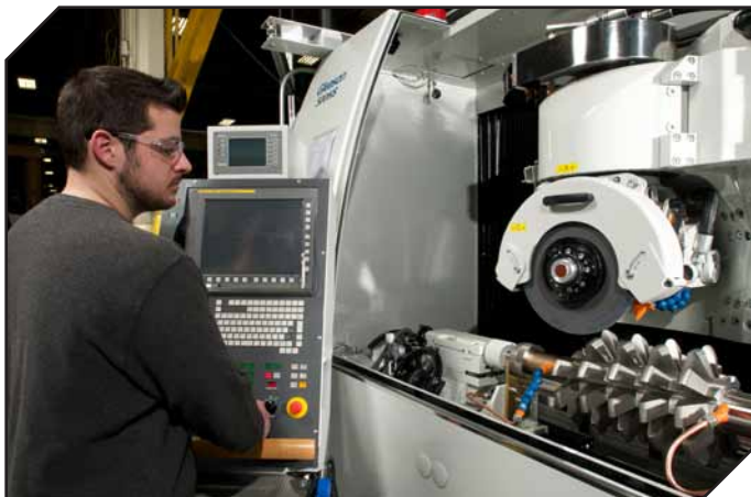
New grinding machines and processes help produce finishing hobs with AGMA Class AA accuracies, precision ground with any desired profile or special involute modification.
