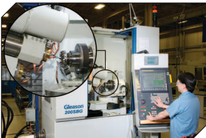
The SBG (solid blade grinder) machine performs one-stop blade grinding on Gleason solid body bevel gear cutters.
