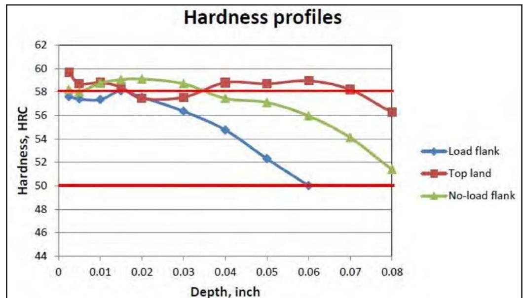
Figure 3 Case hardness profiles of the pinion tooth.
