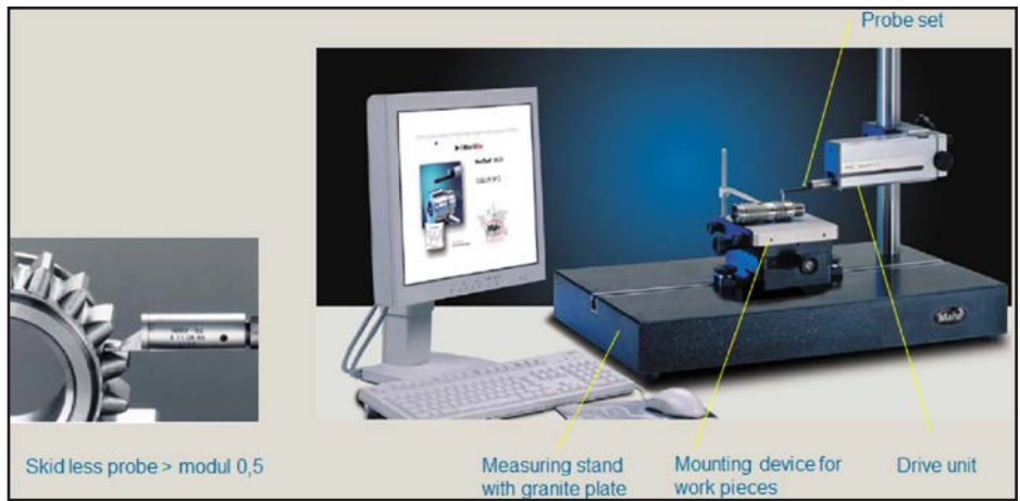
Figure 9 Standard roughness test device — example stationary surface measuring station for gears (Mahr catalog).
