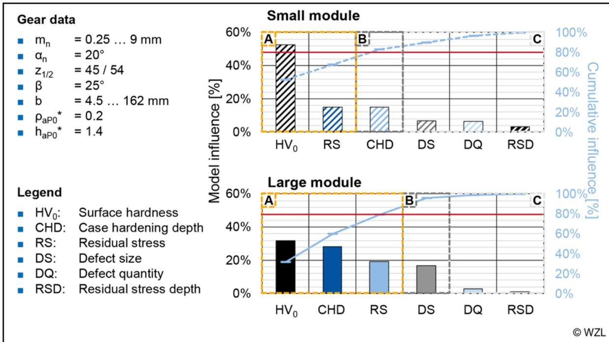
Figure 12 ABC analysis of influence parameters on enhanced weakest link model.
