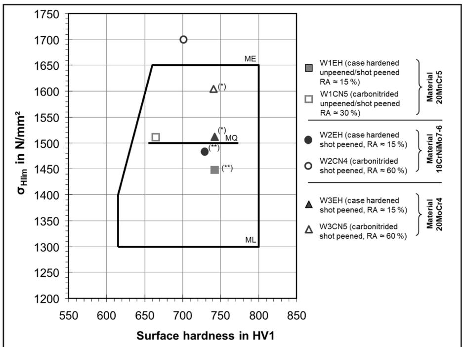
**Figure 2** Classification of the determined allowable contact stress numbers for carbonitrided gears with increased amounts of retained austenite in the standard strength diagram of DIN 3990 (Ref. 4) for case-hardened gears (\*reduced data points, usually about half the data points; \*\*comparison and good correlation with results from earlier investigations (Refs. 14, 20).
