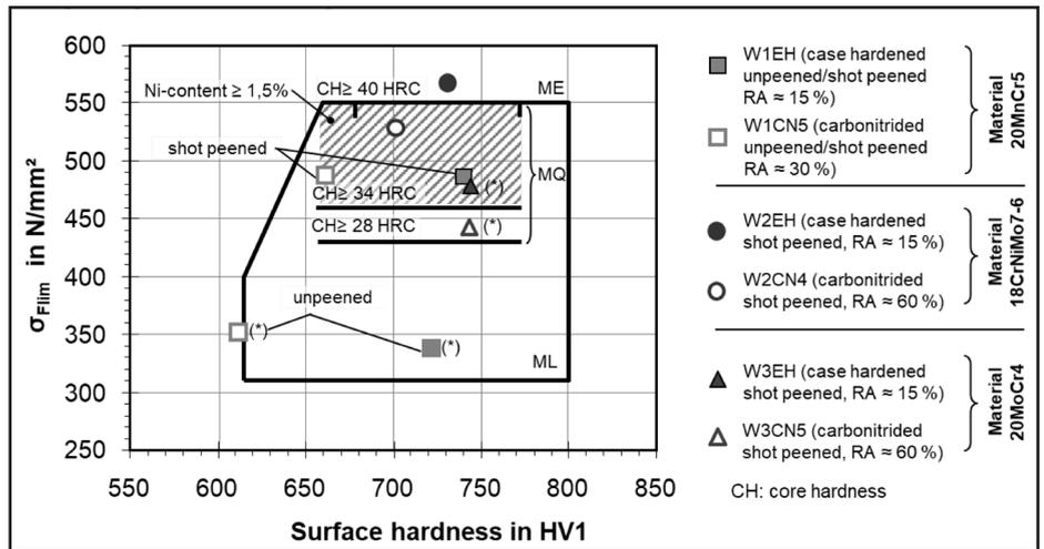
**Figure 1** Classification of the determined allowable bending stress numbers for carbonitrided gears with increased amounts of retained austenite in the standard strength diagram of DIN 3990 (Ref. 4) for case-hardened gears (\*reduced data points, usually about half the data points).
