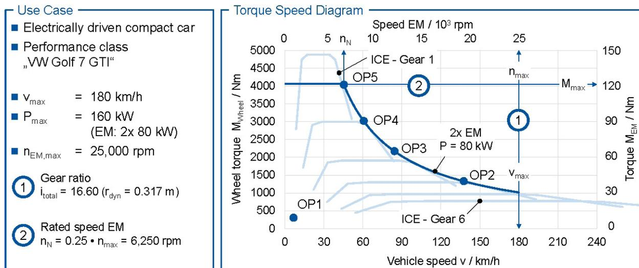
Figure 8 Torque Speed Diagram of the Electrical Machine (EM) and Derivation of Relevant Operating Points (OP)
