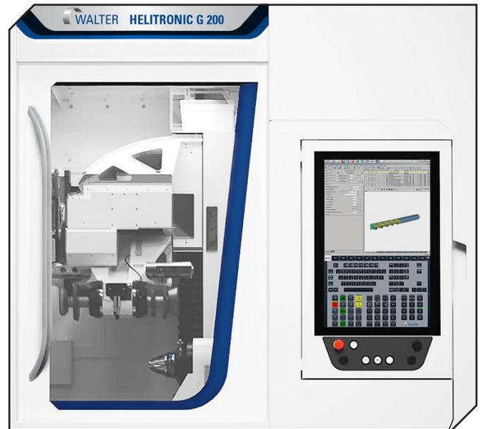
In a floor space of less than 2.3 square meters (24.8 square feet), the HELITRONIC G 200 offers tool grinding and re-sharpening of rotationally symmetrical cutting tools ranging from 1 to 125 mm (0.039" to 4.92") in diameter with a grinding wheel up to 150 mm (5.91"). The HELITRONIC G 200 can accommodate a maximum tool length of 235 mm (9.25") and a tool weight of up to 12 kg (26.45 lbs).
