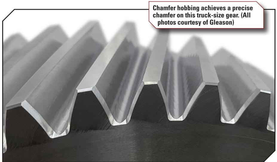
Chamfer hobbing achieves a precise chamfer on this truck-size gear. (All photos courtesy of Gleason)
