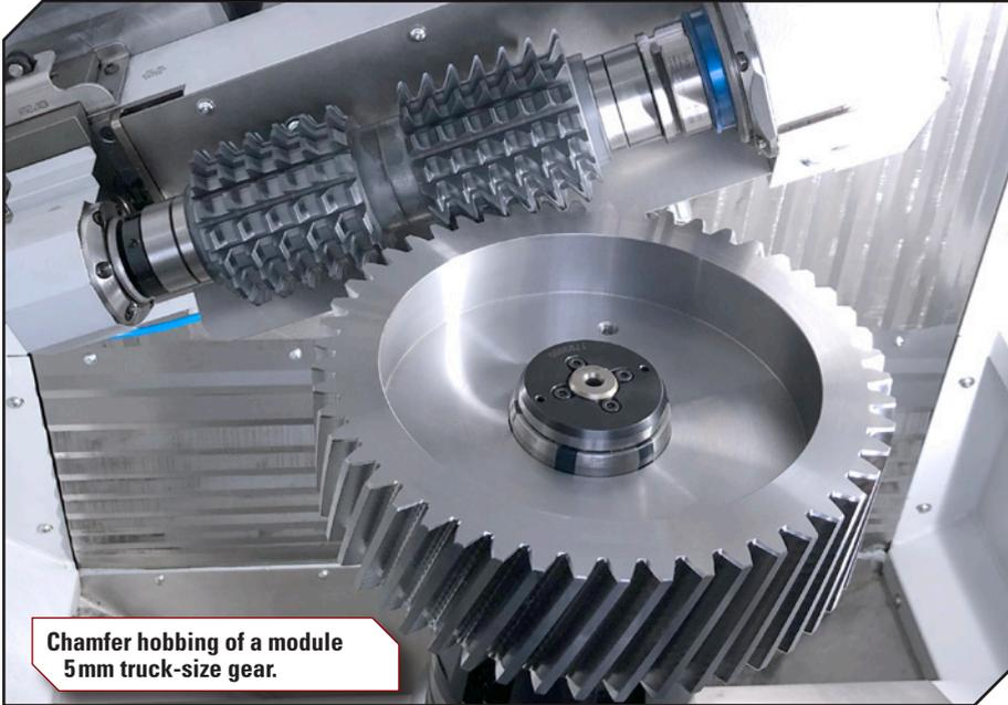
Chamfer hobbing of a module 5mm truck-size gear.
