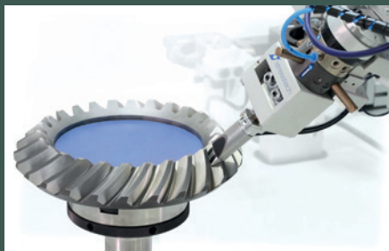
Figure 5—BHN-Testing of gears. (Source: Stresstech GmbH)
