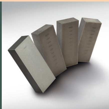
Figure 2—Comparison body NE Test Set. (Source: imq GmbH)
