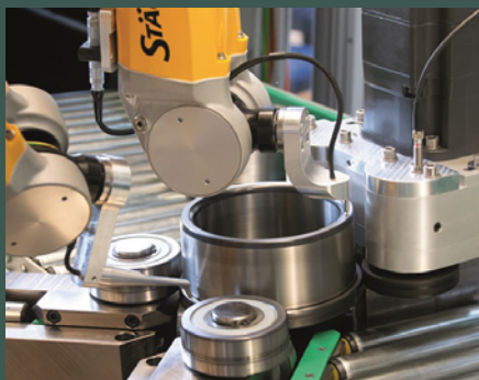
Figure 3—ET testing of a rolling bearing ring. (Source: imq GmbH)
