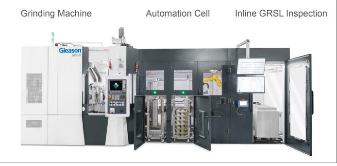
The stacking cell accommodates baskets of various manufacturers and styles and is ideally suited for the autonomous processing of large lot sizes of gears.
