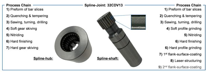
Figure 3—Test-spline joint: process chain.
