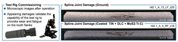
Figure 7—Spline-joint damage.
