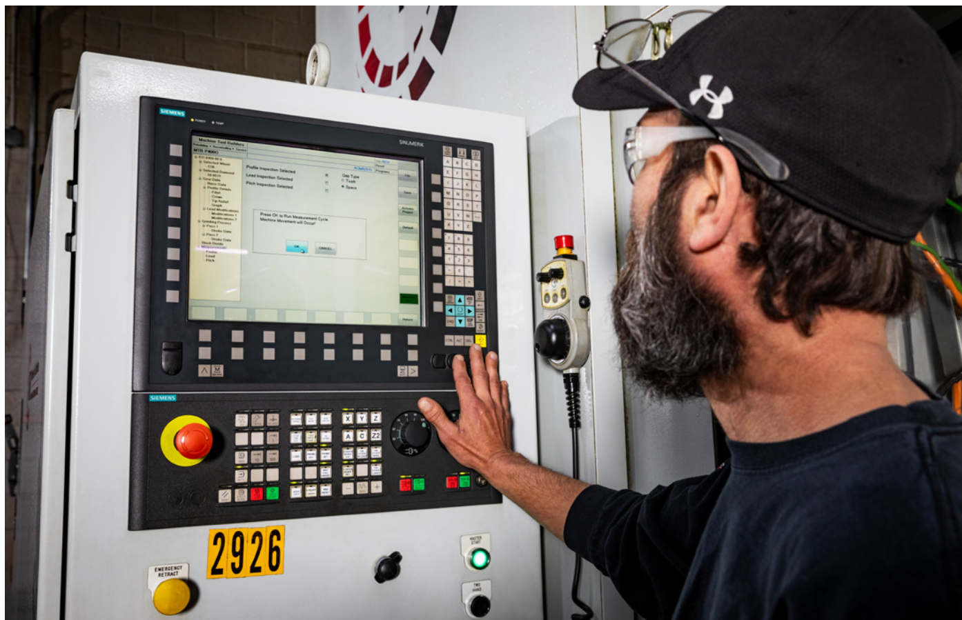
Recontrol to latest Siemens CNC, and MTB's new Form Grinding Conversational Software, combined to empower machine operators and simplify their daily tasks.
