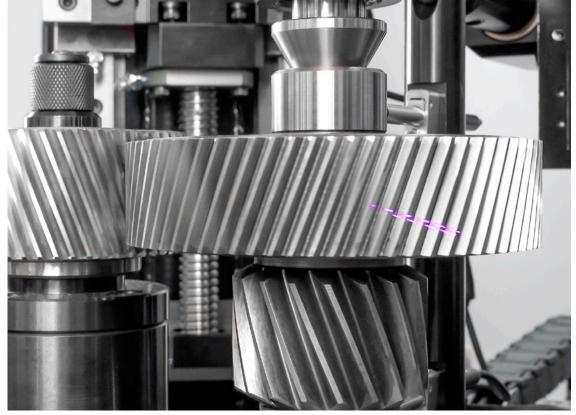
GRSL rolls multiple inspection methods into a single platform: optical inspection of profile, lead, and pitch; DOP and tooth thickness; double flank composite testing; and sophisticated in-process gear noise analysis.
