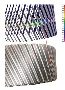
Figure 1—Here, GRSL's point cloud data collection, combined with GAMA software, performs comprehensive noise-related detection and analysis in a fraction of the time of a traditional single- or double-flank roll tester.
