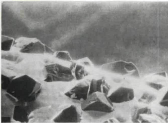
Figure 4 — Micro Photograph of CBN plated form wheel
