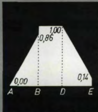
Fig. 2—Traditional load sharing factor for a gear pair with modified tooth profile, designed for high load capacity if the pinion is driver.
