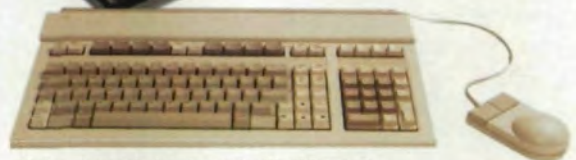
Alpha-numeric keyboard with "Mouse" for one-time entry of part print and tolerance data. "Mouse" permits use of CAD techniques.
