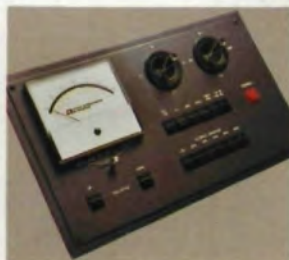
Operator Control Panel for part loading and machine set up. Also provides gage-head meter indication.
