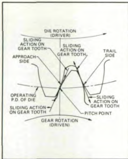
Fig. 4 (left) — Differing flow directions induced by each side of a die tooth with gear roll-finishing.
