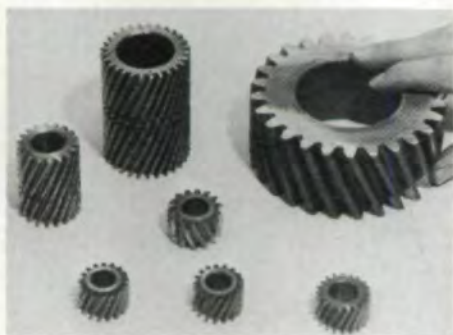
Fig. 9—Gears that have been successfully roll-finished.
