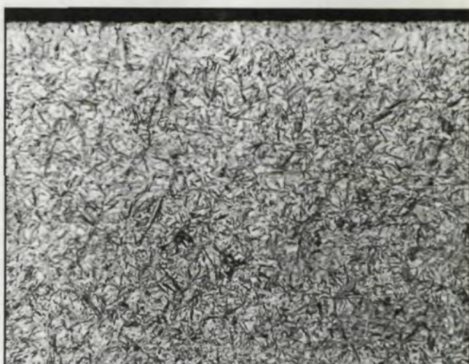
Fig. 10b – Cr-free flank (etched) to show martensite austenite structure. (400X)
