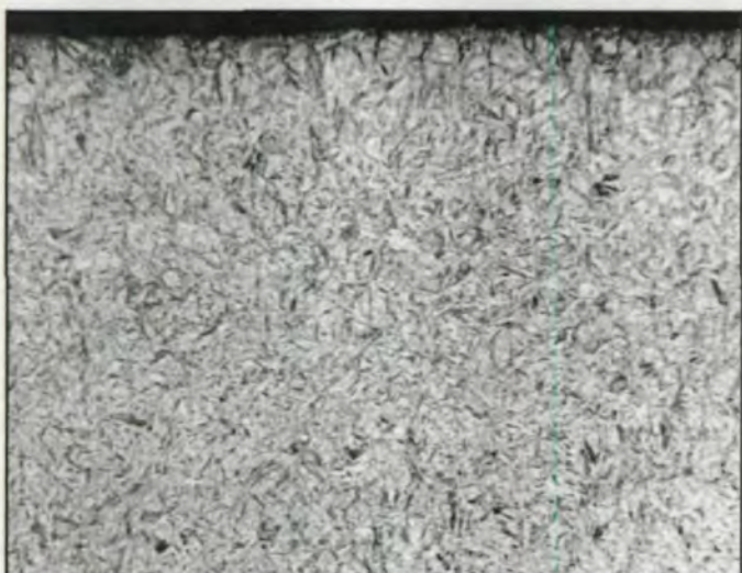
Fig. 10a – 8620 flank in etched condition. Structure is a martensite austenite mix. (400X)
