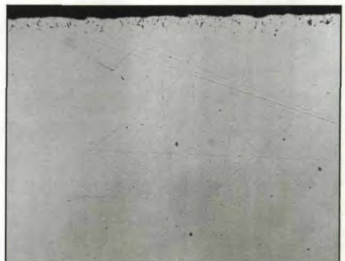
Fig. 8b – (Cr-Free) Flank surface (unetched showing IGO penetration (0.0007).
