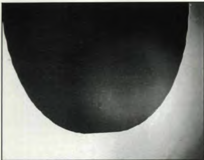
Fig. 14—View showing shape and toughness of root fillet. Specimen #3 — Cr-free alloy 20X.
