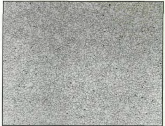
Fig. 11 - Typical prior austenite grain size (heat etch). (100X)
