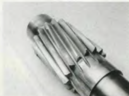
Fig. 8 - The pitting pattern on this helical pinion is the result of a heavy load at one end caused by misalignment.
