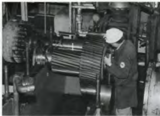
Upper Left: Mobil lubrication engineer Jay Ford performs the yearly gear inspection at Haynes.
