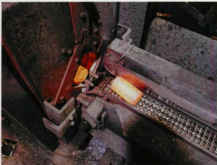
Fig. 5 — Precisely sawn and surface-improved billets are induction heated to about 2,100°F in preparation for the forging process.
