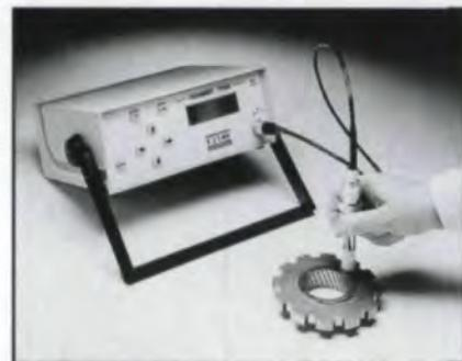
**Portable Hardness Tester With SPC**
