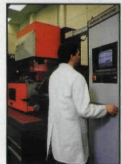
Precision machines, both on and off the track, contribute to Formula One success. Above, the Marlboro-McLaren car with drivers. Below, the Charmilles wire EDM machine used to make transmission gears.
