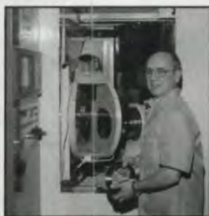
Fig. 4 — Phoenix 450HC-DRY with aerodynamic chip channel.
