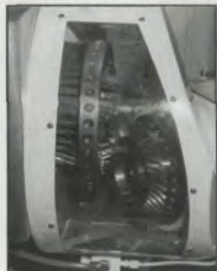
Fig. 1 — View into the work area of a Phoenix machine during continuous-index Power-Dry-Cutting (quarter of plunging depth).
