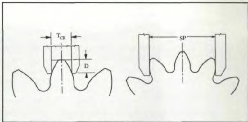
Fig. 3a—Tooth calipers. Courtesy of Van Gerpen and Reece Engineering.
