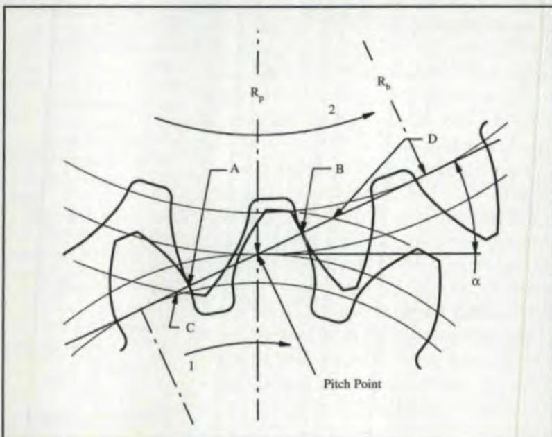
Fig. 5—Base tangent line. Courtesy of Van Gerpen and Reece Engineering.
