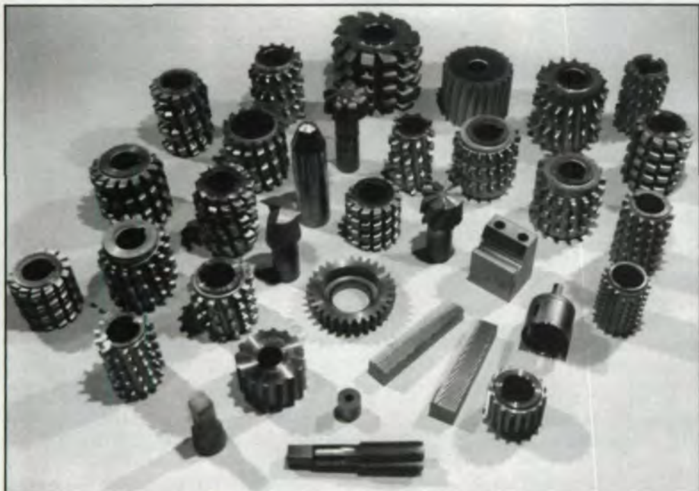
Fig. 1—Coated carbide cutting tools. Courtesy of Ion Vacuum Technologies Corp.
