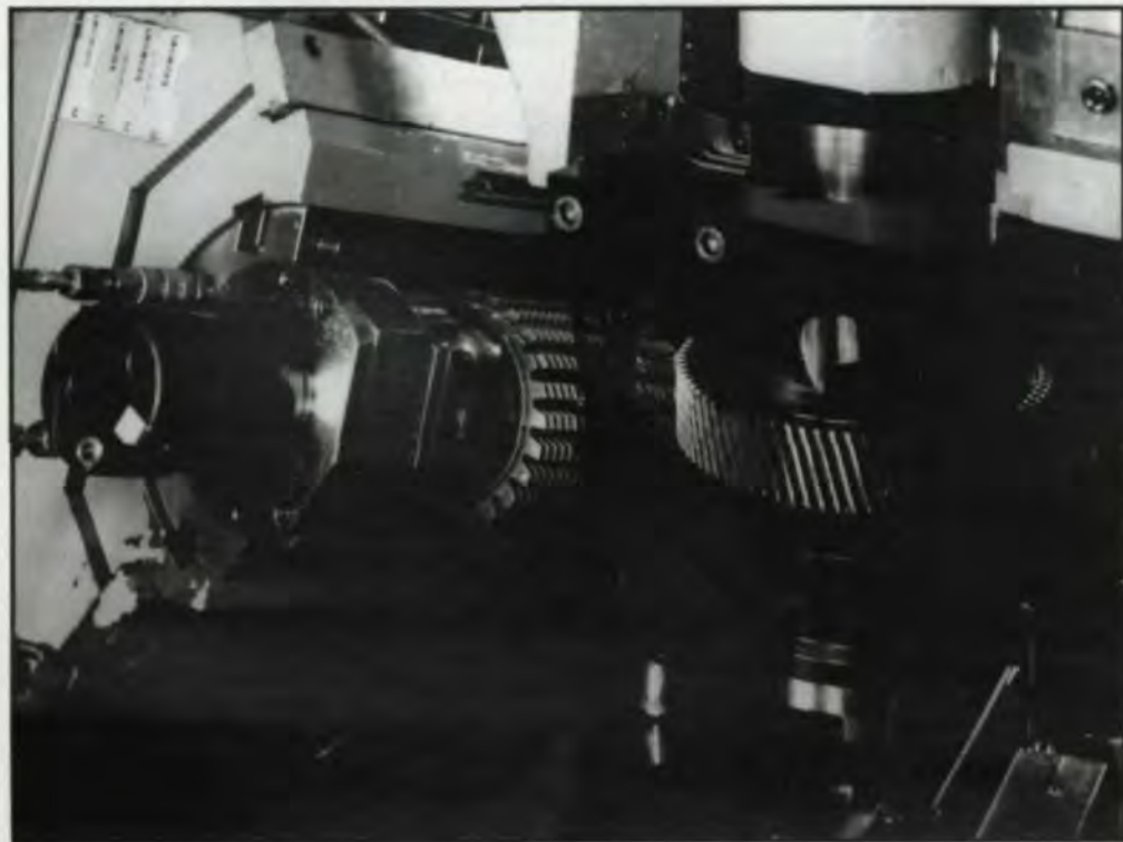
Fig. 2—Wet hobbing of a helical gear. Courtesy of LMT-Fette.
