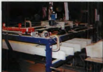
Top: The ice clock used a straight line of gears to achieve a 3600:1 ratio. Middle and Bottom: The homemade CNC router used to make gear templates.
