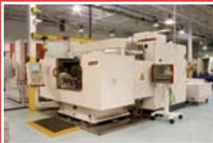
Kapp VUS – Universal Internal/External Form Grinding Machine
