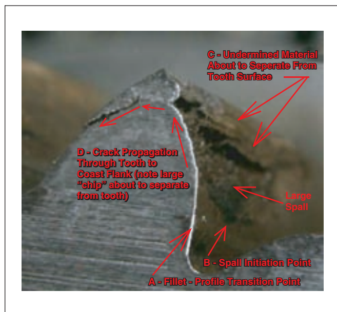
Figure 14—Spall initiation and progression on the pinion tooth (A), enlarged from Figure 11. (Note: Loaded tooth flanks are on the right in this view.)
