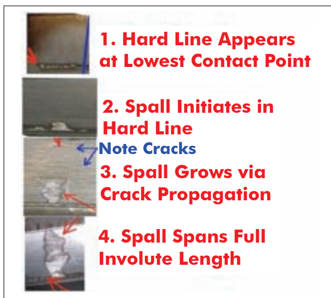
Figure 11—Typical spalling failure progression.
