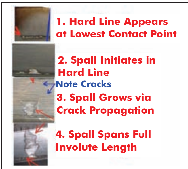
Figure 11—Typical spalling failure progression.
