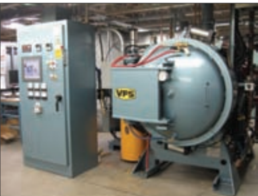
Ipsen's HIQ2624-10 horizontal internal quench vacuum furnace shipped to a customer in the Northeast.
